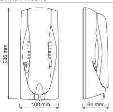
The door phone **Ref. 1133/10** has the same features as Ref. 1133. The only difference is the key on the handset. This key connects the speech wires and must be held pressed for the entire duration of the conversation.
