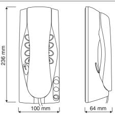
The **Ref. 1133/12** door phone has the same electrical and dimensional features as the basic door phone. It is equipped with:
